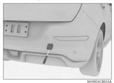
Screw the towing hook into the hole and tighten it clockwise to ensure that it is installed securely.
