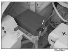
> in the engine compartment fuse box
