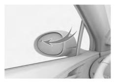
The warning lights are on the surface of the left and right side mirrors.
