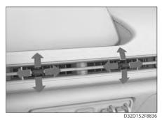
Move the slider in the middle of the outlet vent to adjust the direction of airflow. Move  $\boxtimes \Leftrightarrow$  the slider  $\Rightarrow \boxtimes$  in the direction towards the right hand closed symbol, once it reaches the limit the vent will close.
