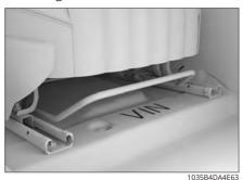
> On the vehicle identification plate below the right C pillar catch.
