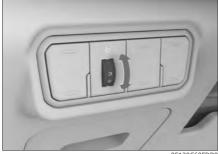
The height of the headlamp beams can be adjusted to take account of the number of passengers and the load in the vehicle.
