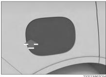
When the driver's door is unlocked, press the charging port cover at the end nearer to the vehicle's rear to open.
