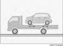
Secure the vehicle in place when using a flatbed tow truck
