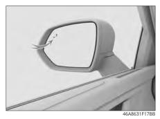
The alarm light is located on the left and right side mirrors.
